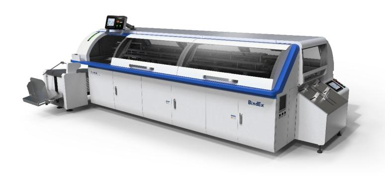
ECOBINDER is a fully automated 5-clamp perfect binder. Except for the cover size which needs to be manually entered on the touch screen, the book thickness data is automatically collected by the automatic thickness measuring device. It is an idea equipment for flexible and quick binding of small and medium book quantities.
