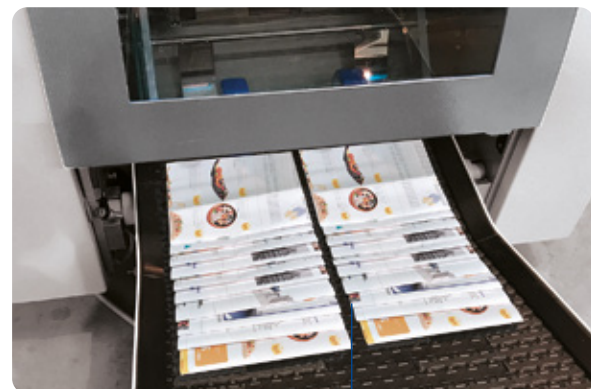
A centre-knife may be easily installed to allow 2-up production of small format booklets
